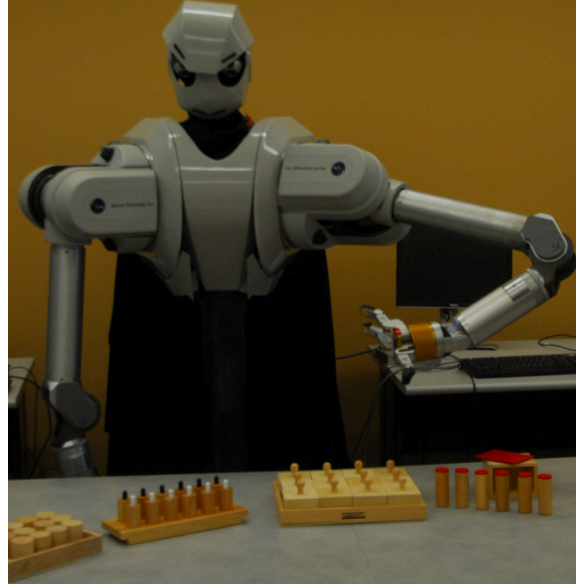
Figure 3.1: The upper-torso humanoid robot. The robot is shown here with some of the Montessori objects that were used in the experiments described in Chapters 4 and 5.
