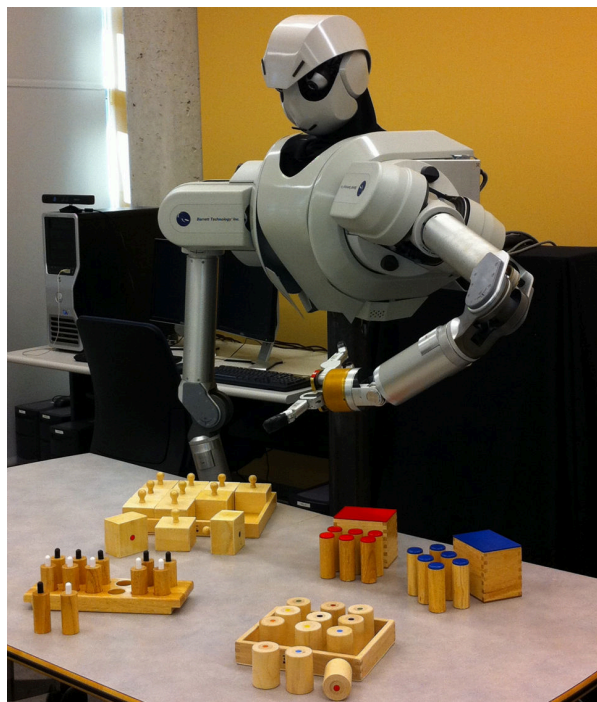
Figure 4.1: The robot and the four Montessori matching tasks that were used in the experiments. In clockwise order, the four tasks were: sound cylinders, weight cylinders, pressure cylinders, and sound boxes.
