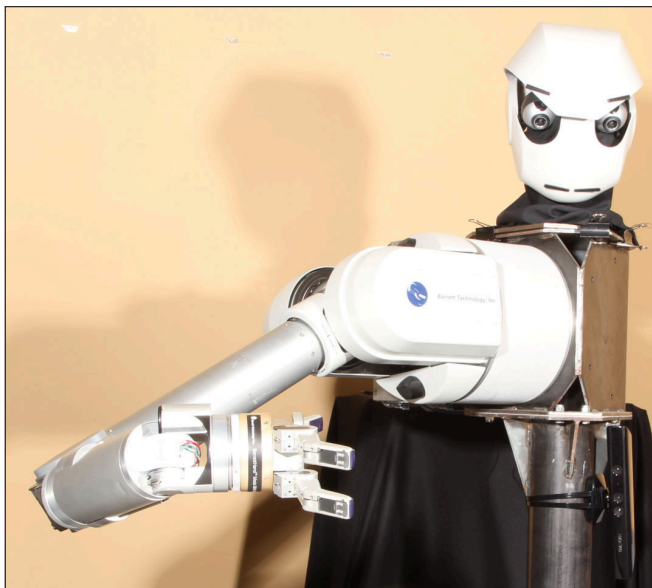
Figure 6.1: The robot used in these experiments. It is shown here with only its right arm as the left arm was temporarily removed for maintenance when these experiments were performed. The Microsoft Kinect camera is mounted on the lower part of the robot's torso.
